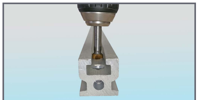
... Countersinking holes on the inside with special countersink
