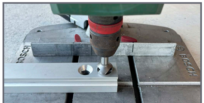
... Lower holes on the outside
