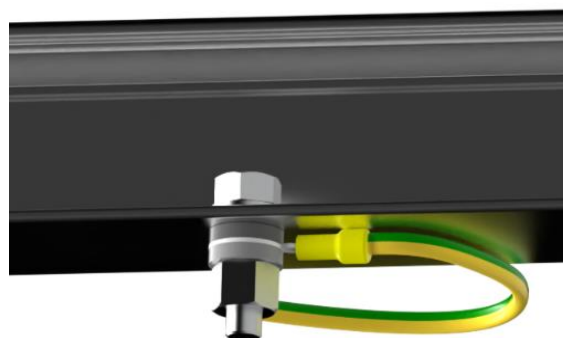
Fig. 11 Grounding of PV modules
